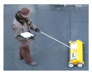
**Concrete & Masonry**: Detection of embedded objects – rebar and conduit in concrete, wall ties and truss mesh in masonry – is not inhibited by the cold. The only concern is battery life, so we bring spares and chargers to the site. Impact measurements such as thickness with impact-echo, strength with rebound hammer, and void/delamination testing with sonics or ultrasonics are also not affected by the cold.
